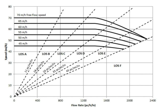
Figure 10. Multilane Highway Segment Speed-Flow Curves
