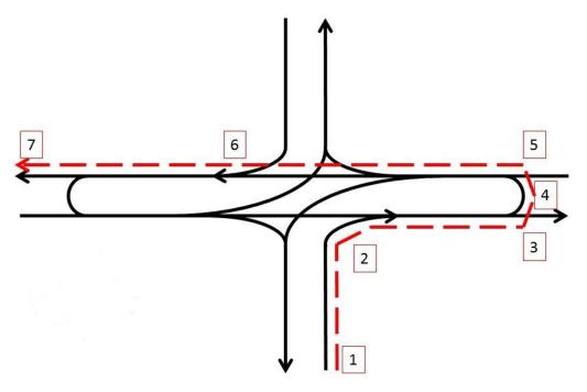
Figure 24. Example of experienced travel time at an RCUT intersection Source: HCM
