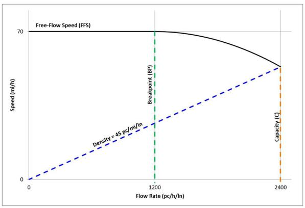
Figure 8. Unified speed-flow equation
