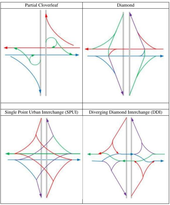
Figure 22. Ramp Terminal Forms
