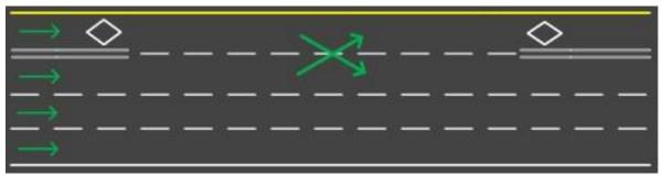
Figure 11. Weaving in a Managed Lane Access Segment
