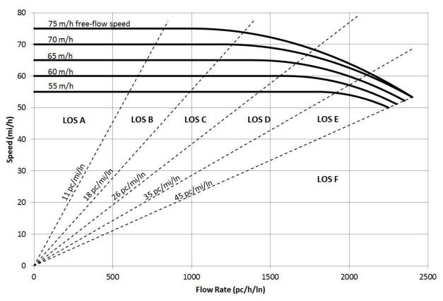
Figure 9. Basic Freeway Segment Speed-Flow Curves
