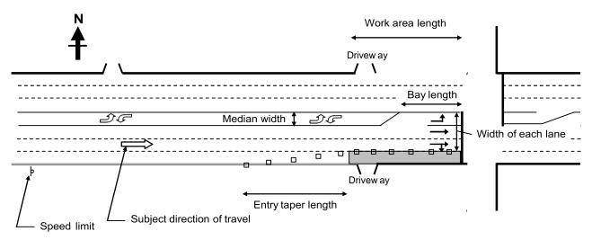
Figure 20. Work zone presence at approach to signalized intersection
