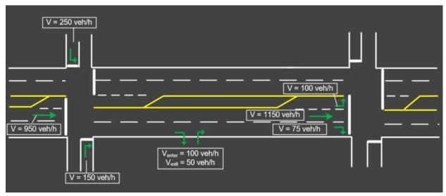
Figure 18. Right-turn-on-red vehicles incorporated into volume-balancing method
